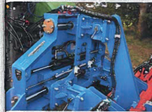
Three sizes of mounting carriage are available to suit different working widths. The version pictured includes hydraulic steering by double-ended ram, and positioning is monitored by a potentiometer directly below the ram.
