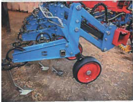
The pictured unit is equipped with a hydraulic lift ram which is part of a section control system.
