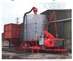
to the Magna range is the Duax heat core – heat retaining bricks that ensure a more even and consistent drying temperature with the added benefit of saving up to 10% on diesel costs.
