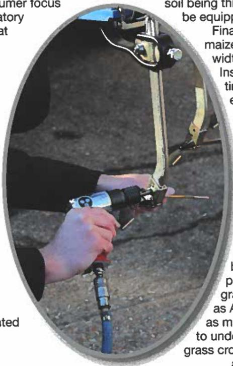
*The changeover of shares can be done quickly and easily using pneumatic tools.*
