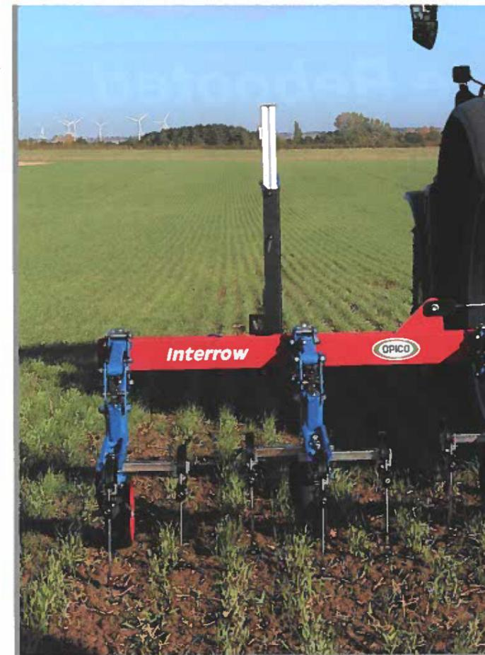
*Up to eight cameras can be fitted, along with a steerage headstock for automatic sideshift.*
