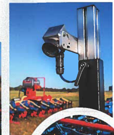
A Muller section control system, similar to that on sprayers, can lift parallelograms out of work as required
