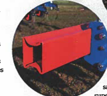
Above: This bespoke steel tube ensures tools can be securely clamped on to the cultivator
