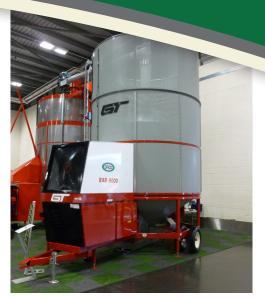
Supplied as standard with 38" custom built, in line centrifugal fan (74 dba). Unique self diagnostic electronic Grain Guard control. Centralised greaser location. 60 ton an hour 12" diameter central auger 8" diameter loading auger with full length, 9ft 10" (3m) loading hopper (50 ton an hour loading capacity). LP Gas fired burner. Epoxy powder coated outside sheets. Adjustable jacks, 4 tyres, grain sampler. Horizontal discharge auger. 3-phase electric drive.
