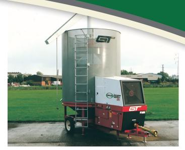
Supplied as standard with 33" custom-built, in-line centrifugal fan (74 dba). 8" diameter loading auger (50 ton an hour loading capacity). Full length 9ft 10" (3m) loading hopper. 60 ton an hour 12" diameter central auger. Centralised greaser location. Epoxy powder coated outside sheets. Adjustable screw jacks. Grain sampler, grain cleaner. Grain pressure splitter pelmet. LP gas fired burner. Grain Guard Monitor control system.
